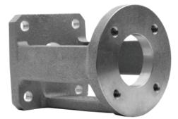
Gas Engine Adapter - PEM-F Flange (inches) XBF Pump Mounting XAJ M Face to MAX XAK Mounting Holes Coupling Pump Pilot Pump Bolt Inside Part No. (NC) Clearance Туре Flange Circle Face 6048 USAF 4F17 4 Bolt 2.63 2.84 1.78 5/16-18 4.50 3.38 6049 SAE AA 2.81 3.25 2.00 3/8-16 4.50 3.38 2 Bolt 6061 SAE A 2 Bolt 2.81 4.19 3.25 3/8-16 4.69 3.38
