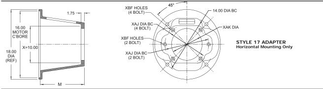
If your pump is not listed or is a non-standard pump, contact us for special machining and/or information. Not all pump mounting holes are supplied on every adapter.
